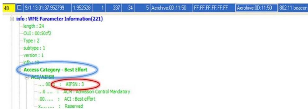
Figure 6 shows a Beacon frame that includes the AIFSN value for this BSS. These values can be found for each AC in the EDCA Parameter Set Element within a Beacon frame. In Figure 6, a blue highlight shows the Best Effort AC and the red highlight shows that the AIFSN is currently set to 3, the default setting. The AIFSN value determines the duration of the AIFS[AC], as we will discuss in a later section, titled *Calculating an Interframe Space*.
