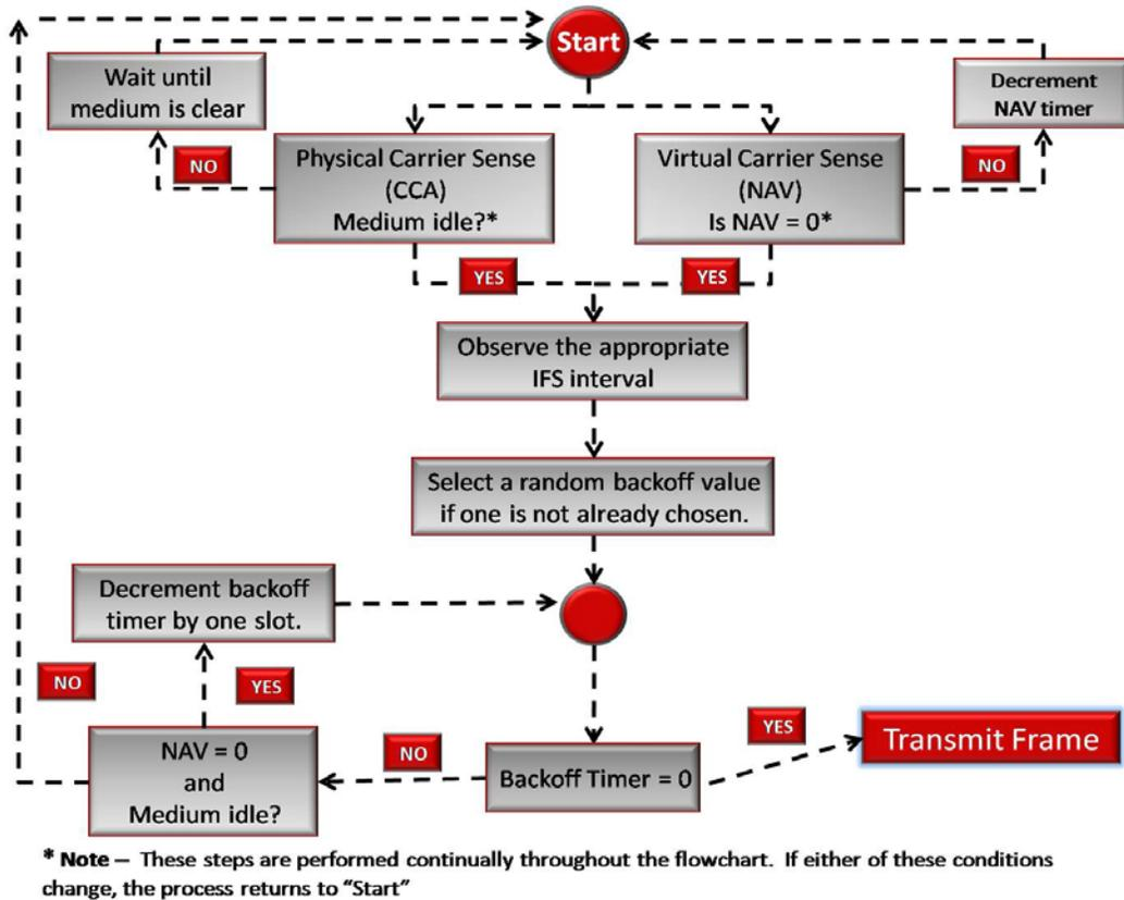
Figure 3 provides a graphical perspective of the steps described previously. Despite the figure's simplicity, it should help readers to organize the flow of 802.11 arbitration. A detailed analysis of these functions follows.
