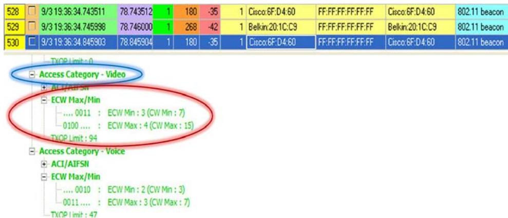
The fixed DCF aCWmin and aCWmax values are shown in Figure 12 and the default EDCA aCWmin and aCWmax values are shown in Figure 13. Comparing the values shown in Figure 11, you will notice that both the video and voice ACs in this Beacon frame represent the default CW parameters for the EDCA function.
