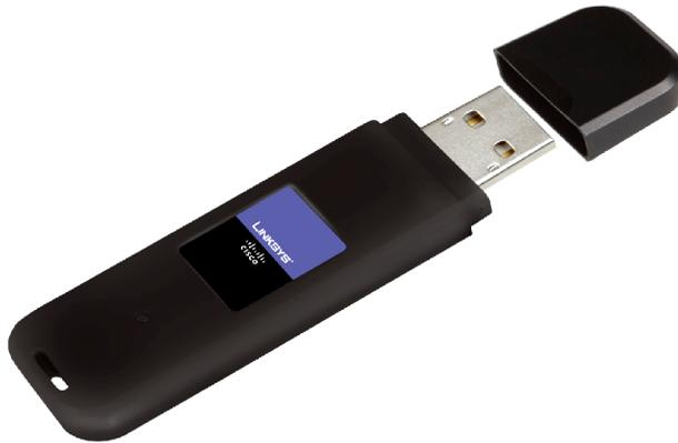
The Linksys WUSB600N wireless client adapter is dual-band 802.11n capable, has a Ralink chipset, and is supported by the OmniPeek MultiChannel Aggregator Plug-in. Having a USB 2.0 interface allows for use of multiple simultaneous adapters on the same laptop PC. Special WildPackets drivers are required for this adapter to operate properly with OmniPeek Enterprise and the MultiChannel Aggregator Plug-in.
