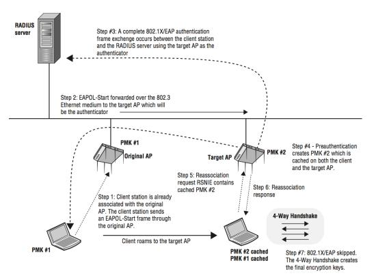
A client station can use preauthentication to establish a new PMKSA with an AP prior to roaming to a new target AP.
