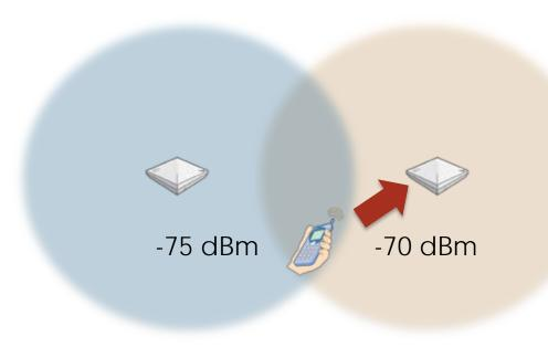
Clients make the roaming decision Based on factors such as RSSI or SNR The client sends a frame called the reassociation request frame, to start the roaming procedure.
