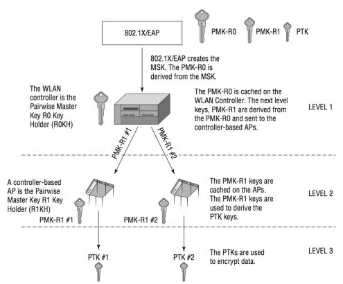
• The access points are the key holders for the PMK-R1 keys.
