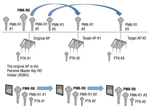
• The PMK-R1 keys are cached on the target APs, which are the key holders for the PMK-R1 keys.
