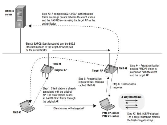
The purpose of the new 802.1X/EAP authentication is to create a new PMKSA relationship with a new target AP where the client might roam.
