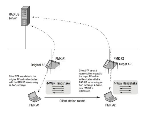
802.1X/EAP authentication can take 700 milliseconds (ms) or longer for the client to authenticate.
