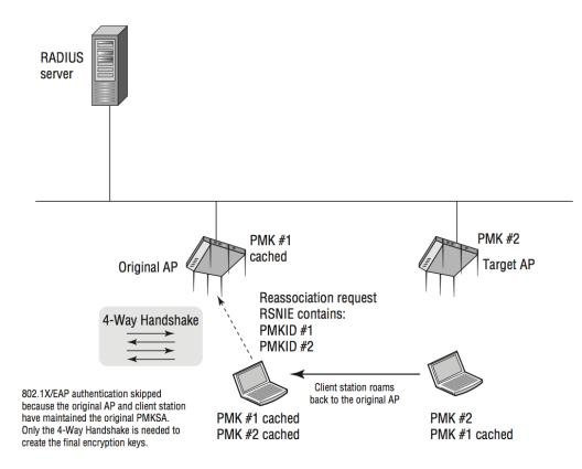
• The 802.11-2012 standard states "An AP whose authenticator has retained the PMK for one or more of the PMKIDs can skip the IEEE 802.1X/EAP authentication and proceed with the 4-Way Handshake."
