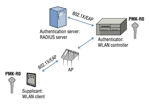
The first time a client station enters a mobility domain, the client will associate with an AP and perform an initial 802.1X/EAP authentication.
