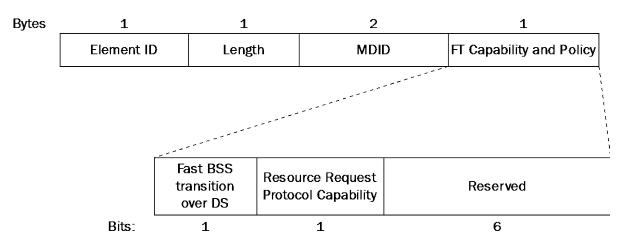
The FT capability and Policy field is used to indicate whether overthe-air or over-the-DS fast BSS transition is to be performed.
