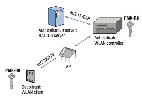
• The first-level pairwise master is called the PMK-RO key and is sent to the authenticator and the WLAN client.
