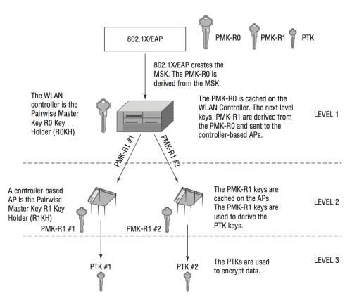
The PMK-R0 is created and cached on the WLAN controller. The WLAN controller is the key holder for the first-level key.
