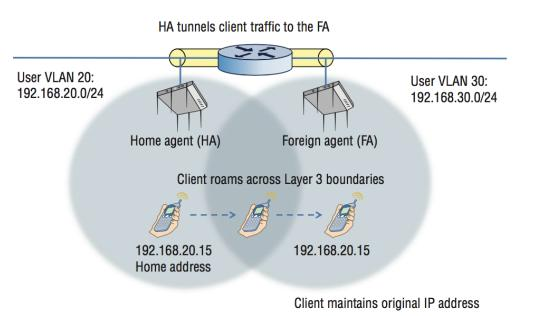
The only way to maintain upperlayer communications when crossing Layer 3 subnets is to provide a Layer 3 roaming solution that is based on the Mobile IP standard.
