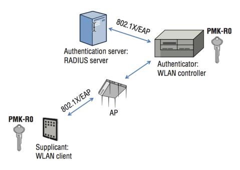
The various levels of FT keys are derived and stored in different WLAN devices depending on the WLAN architecture that has been deployed.
