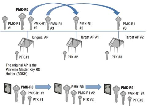
• The second-level PMK-R1 keys are derived from the PMK-R0 and sent from the original AP to other target APs over a secure channel.
