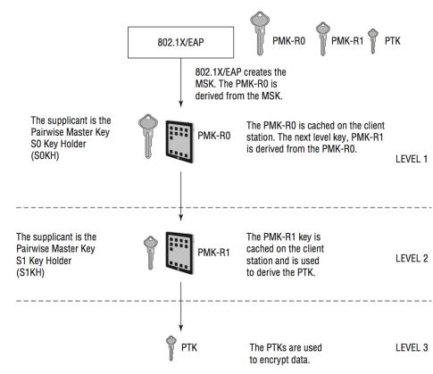
The various levels of FT keys are also derived and stored on the client station.
