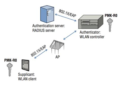
• FT uses the 802.1X/EAP exchange to create the master session key which seeds a multi-tiered key management solution.
