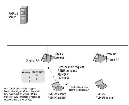
• The client does not need to re-authenticate and create a new PMK because the original PMK still exists.
