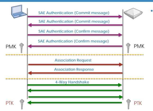
Once the PMK is created and the association process completes, the AP and the client can then commence a 4-Way Handshake to create a pairwise transient key (PTK).
