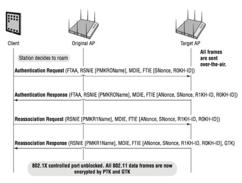
An FT protocol frame exchange is used to initiate the roaming exchange and create dynamic encryption keys.
