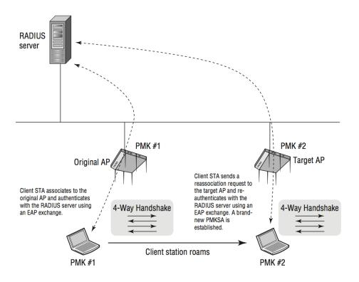
Without any type of fast secure roaming mechanism
