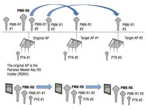
The 802.1X/EAP exchange creates the master session key (MSK). The MSK is used to create the first-level master key, PMK-R0.
