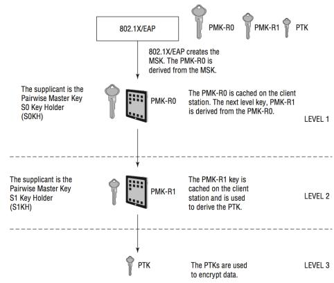
The client station derives the second-level key, PMK-R1, from the PMK-R0.
