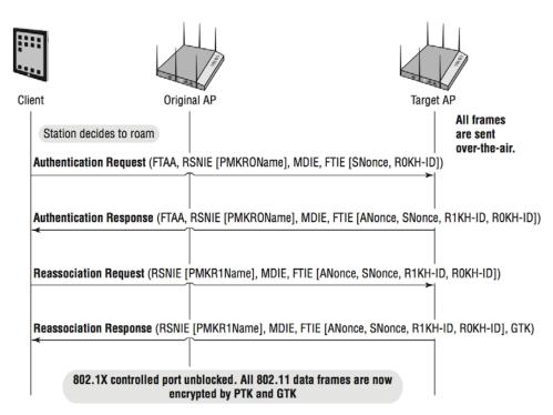
The FT process defines a more efficient method that effectively combines the initial Open System authentication and reassociation frames with the 4-Way Handshake frames.
