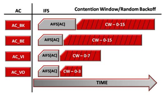
FIGURE 14 – Conceptual comparison of AIFS and CW for each AC
