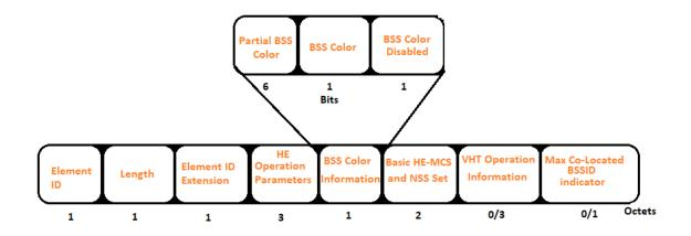
And by looking to the frame bits of the BSS Color Information you can find that it is an identifier for a number between 1 to 63, and this can identify for 63 Basic Service Sets. Each identifier number can discriminate one BSS radio from another radio on the same channel by the color number (1-63), but if the color number is identical to another BSS here, we call it an intra-BSS frame, and for the different BSS color then stations will consider in an inter-BSS frame.
