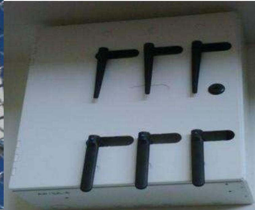
Mount the box horizontal and extend the antennas down and not right up against the metal enclosure
