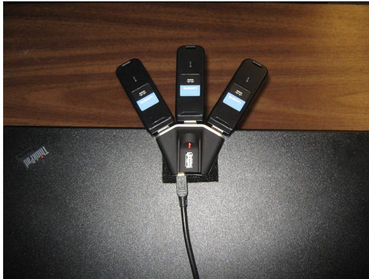
This picture shows the laptop-mounted USB hub with three WUSB600N adapters attached. Even with the three wireless adapters mounted, a small strip of Velcro holds the hub securely. It is best to mount the top edge of the USB hub to the top edge of the back of the laptop screen. This prevents the laptop screen from blocking RF signals. We have cut the Velcro that attaches directly to the USB hub to fit with no overlap. On the laptop, you can just have a nice square piece of Velcro.
