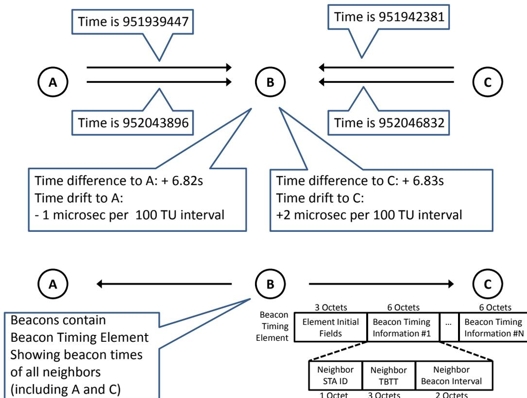
Anti-collision mechanism for beacon frames, MBCA (11C.12.4)
