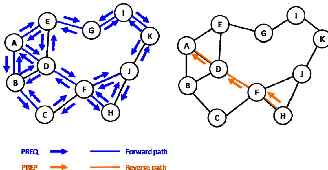
A station on the path (for example D) will remember that it is on the best path from A to H (identified by the components of the PREQ), and that the next hop to H is F, and the precursor (next hop back to A) is A itself.
